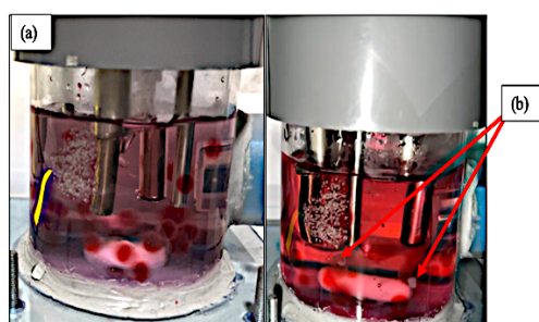
Figure 5 Mixing performance by fabricated magnetic stirrer mini bioreactor showing (a) beads distribution, and (b) beads fragment impact from the uncontrollable stirring.
